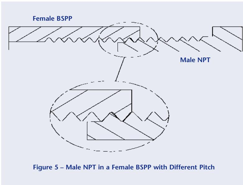
Another tapered thread is the British Standard Pipe taper, or BSP, covered by British Standard 21. BSP thread is commonly used for low pressure plumbing, but is not recommended for medium and high pressure hydraulic systems. This form uses the Whitworth thread with an angle of 55° and a 1 in 16 taper. It is not interchangeable with the American NPT thread, though at the 1/2" and 3/4" size, they both have 14 threads per inch.
