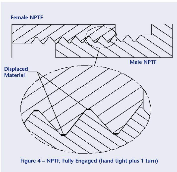
Figure 4 – NPTF, Fully Engaged (hand tight plus 1 turn)
