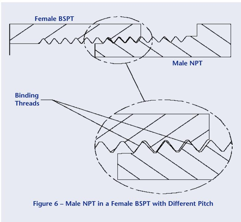
Figure 6 shows an NPT tightened into a BSPT. The BSPT being wider at the opening will allow the NPT thread to engage further, but pitch difference eventually causes a binding of the threads. Pitch and thread angle differences will allow spiral leakage.
