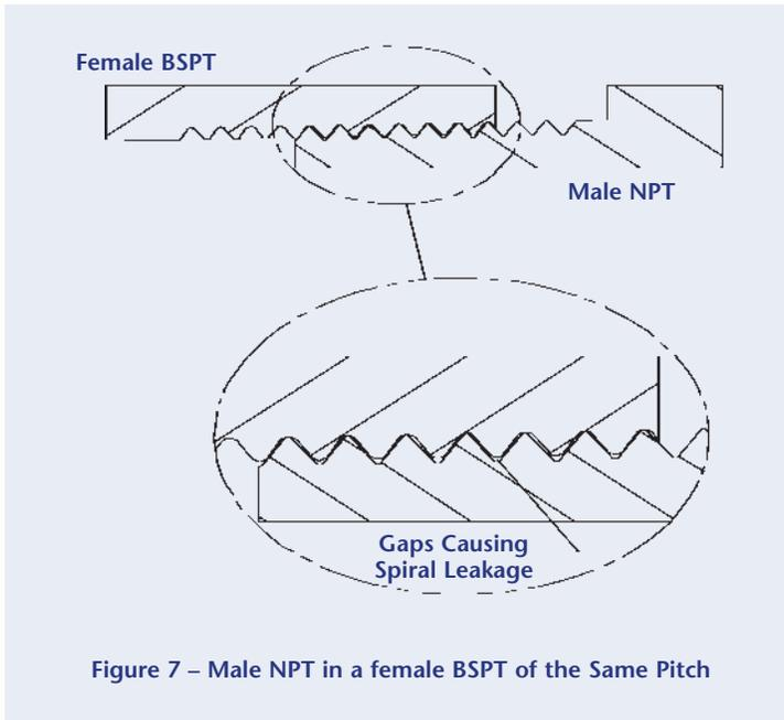
Figure 7 – Male NPT in a female BSPT of the Same Pitch
