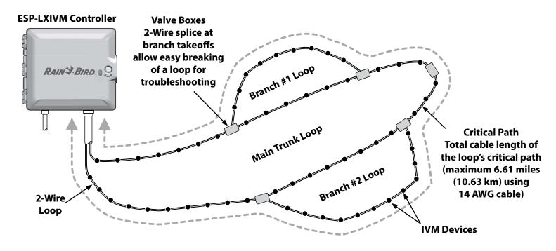
2-Wire Loop Pattern design showing IVM Devices and Valves
