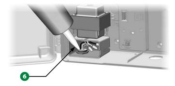
7 Verify that all connections are secure. Then replace the cover of the transformer wiring compartment and secure it with the screw.
