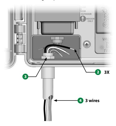
**5** Using supplied wire nuts, connect the wires accordingly.
