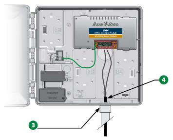
5 Using a thin blade screwdriver, connect the two wire ends to a set of large 2-Wire path terminals on the ESP IVM 2-Wire Interface Module. When finished, tug gently on the wires to make sure the connections are tight.
