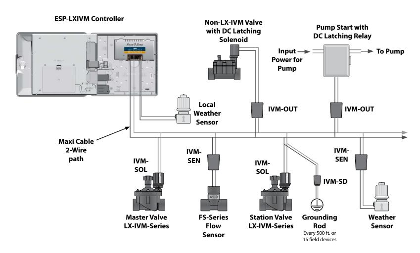
**ESP-LXIVM 2-Wire Control System showing IVM Devices connected**
