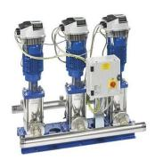
Variable speed booster sets assembled with two up to four pumps. The frequency converter (hydrovar) is installed on each pump. The pumps used are the eSV model.
