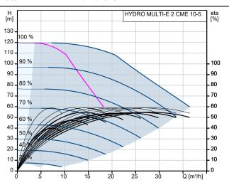
Losses in fittings and valves not included Pumped liquid = Water Liquid temperature during operation = 20 °C Density = 998.2 kg/m³
