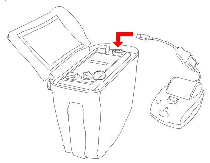
Switch the welding unit on, when the printer is detected the screen below is displayed.
