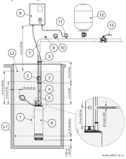
The figure shows a typical installation.
