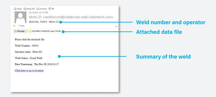
Data files are opened with the CalderSafe Weld Analyser.
