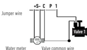
Connect your + S - input to a water meter equipped with a flow sensor as shown above. Use dry contact flow sensors or equivalent. For polarized flow sensors, when wiring, observe the polarization :
