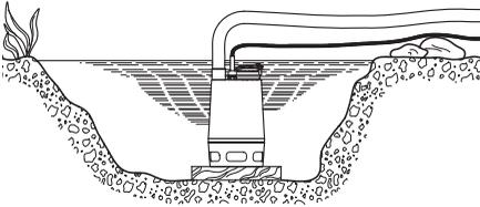
Fig. 2 Place the pump on a plate
