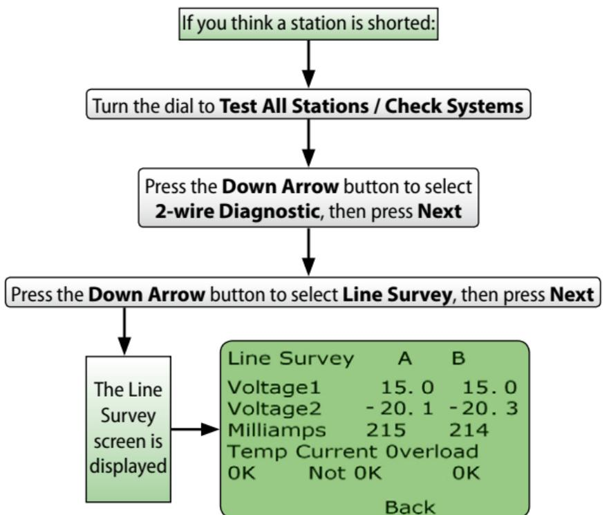
**!** **NOTE:** The Voltage1 reading for a normal healthy system is typically in the +14.0 to +16.0 range for both A and B. The Voltage 2 reading is typically in the -20.0 to -21.0 range for both A and B. The Voltage1 and Voltage2 readings should be approx. equal for A and B. Milliampage (mA) varies with the number of decoders installed and should be approx. equal to the amperage calculations detailed on [page 16](#).
